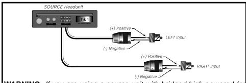
**WARNING:** If you are using a source unit with bridged high powered (or "floating ground") speaker outputs, a suitable high to low level adapter must be used. If you are unsure about your head unit see your local Precision**Power** dealer or call **1-800-62Power**.
